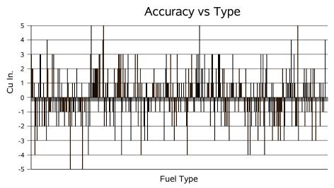
There is no consistency of calibration when comparing fuel types The repeatability does not change with the use of different fuel types. The chart below shows the results on one type of fuel. The results are consistent with any of the fuel types. Essentially no pattern is discernible.
